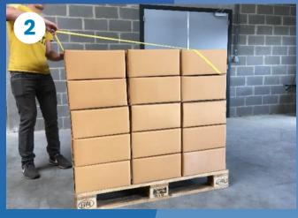
Start stretching the rubber band by placing yourself at the opposite corner of the pallet.
