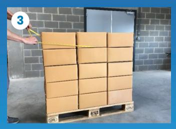
Continue by placing the rubber band on each edge of the pallet. Equalize the tension for an optimal result.
