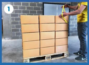
Secure the rubber band by wedging it under one of the cartons to be palletized. Check that the rubber band is well fixed by applying tension.
